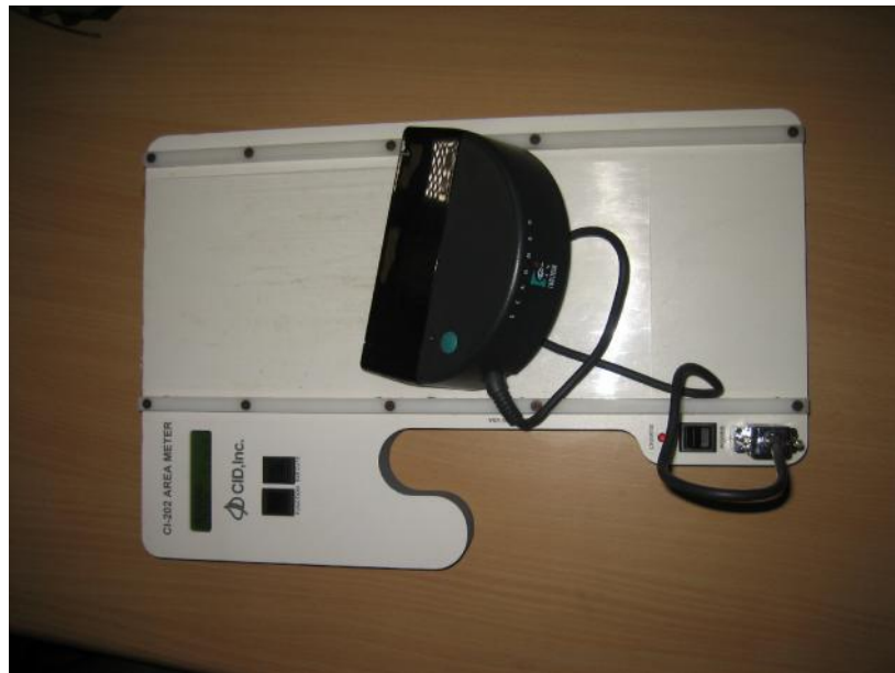
Plate 1: CL-202 Leaf Area Meter CID Inc., Van- couver, USA
