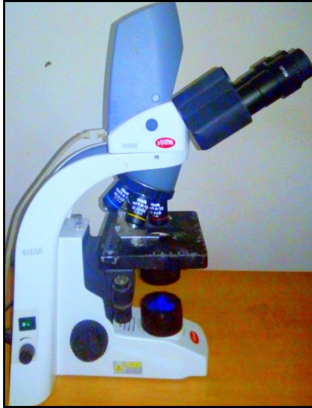
Photograph 4: Digital microscope (Model: Motic, BA-210)
