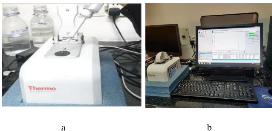
Figure 4. Quantification of DNA through Nanodrop Spectrophotometer (a) DNA sample loading, (b) Graphical result presented DNA concentration and purity.
