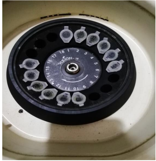
Plate 5. Centrifugation for identifying DNA containing layer
