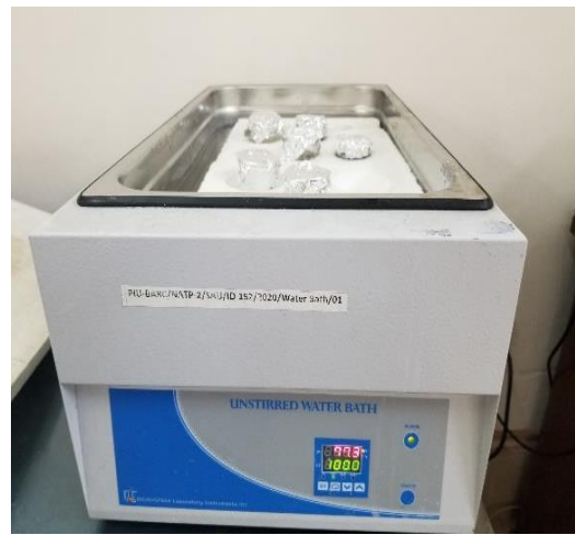
b. Micro beakers in water bath for the estimation of total sugar
