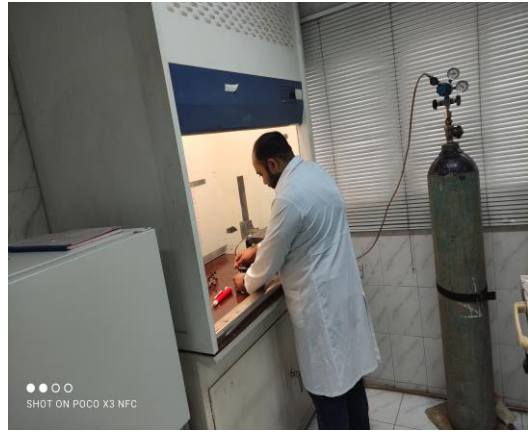
Plate 8. Placing of vial in sample concentrator and drying by N 2 gas
