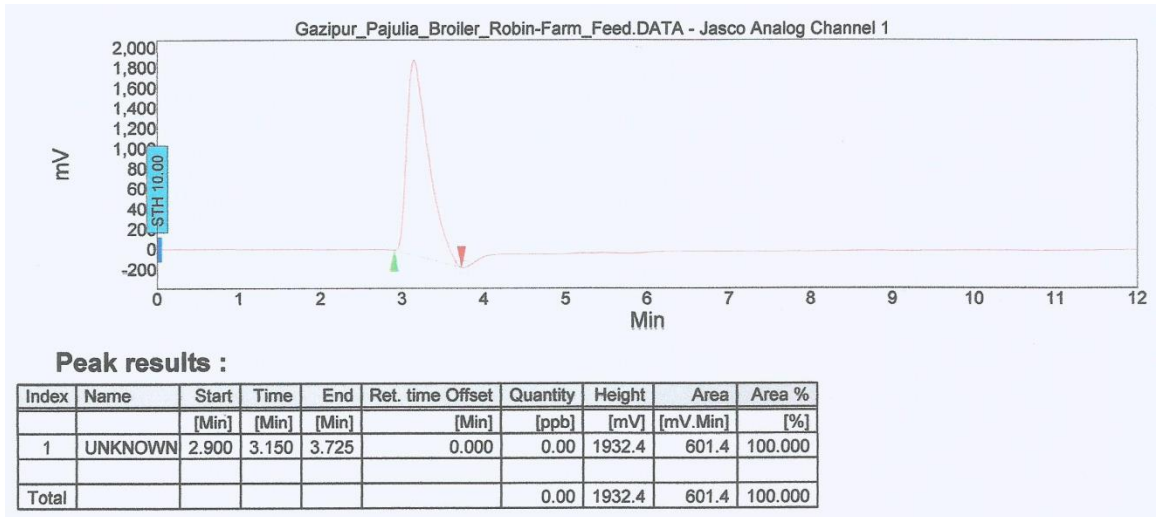
Figure 47. Chromatogram of TC and OTC in broiler feed (sample id GCBCRoF)
