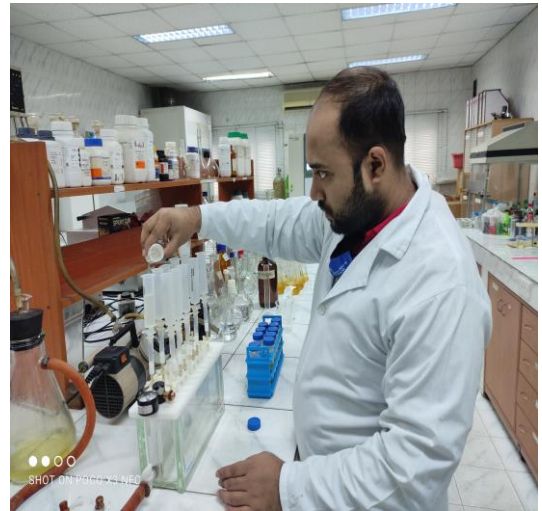
Plate 7. Drain of filtrate sample extract through SPE by using vacuum manifold
