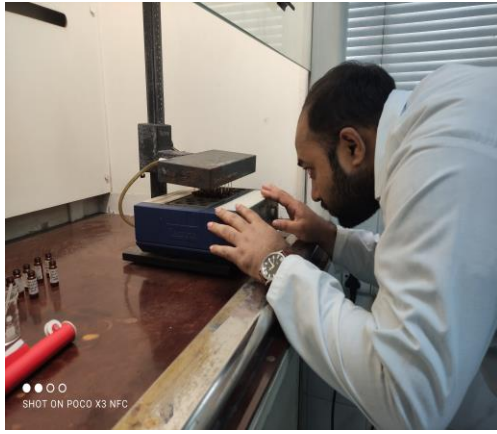
Plate 8. Placing of vial in sample concentrator and drying by N 2 gas
