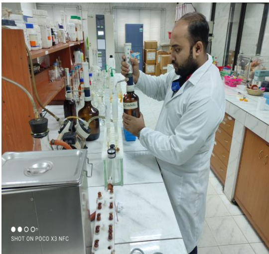
Plate 7. Drain of filtrate sample extract through SPE by using vacuum manifold
