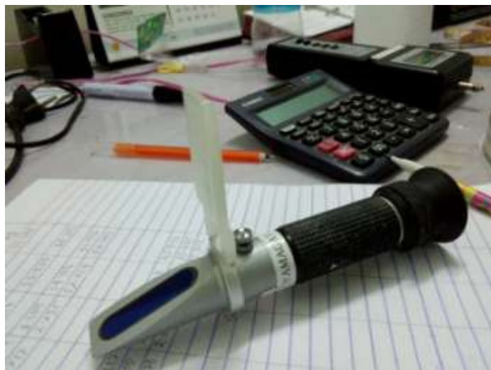
Plate 4. Refractometer for TSS determination
