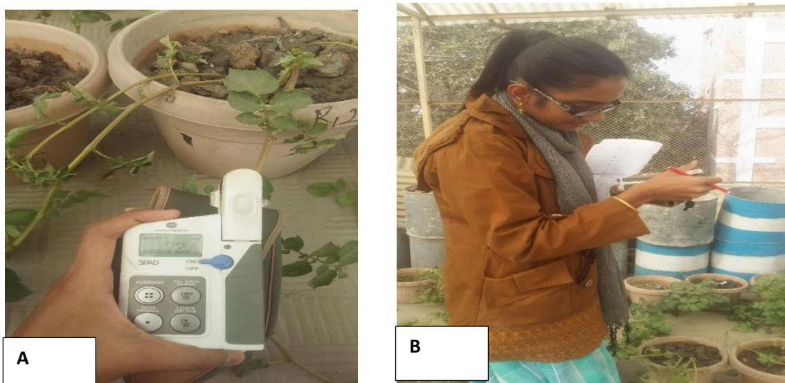
Plate 6. Different types of physiological analysis and data recording A. SPAD-502 plus portable chlorophyll meter B. Determination of chlorophyll content SPAD-502 plus portable chlorophyll meter.
