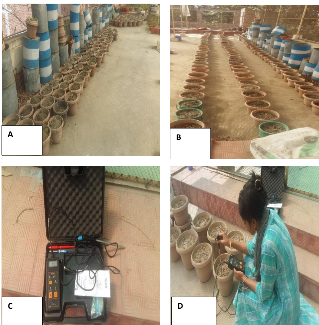
Plate 1. Preparation of pot before sowing A. Filling the pot with soil B. Arranged the pot according to replications C. EC meter to check saline level in soil D. Checking the level of soil salinity.
