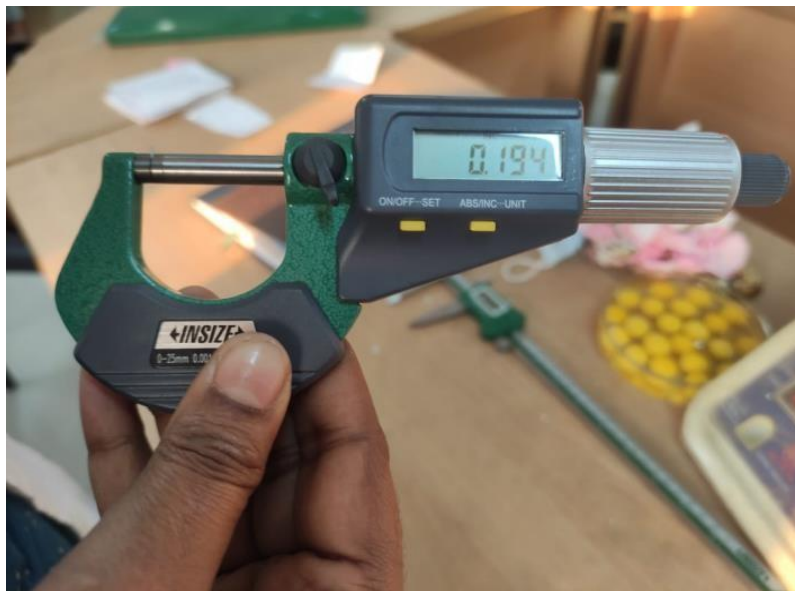
Figure 27. Measuring shell thickness
