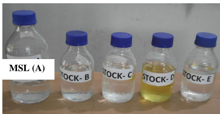
Plate 1: Standard dose of Stock solution-A ( 16.50 \text{ gmL}^{-1} of \text{NH}_4\text{NO}_3 ) and other stock solution B, C, D and E for MS media preparation
