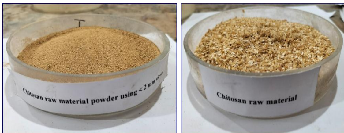
Plate 1: Chitosan raw material and Chitosan raw material powder using <2 mm sieves
