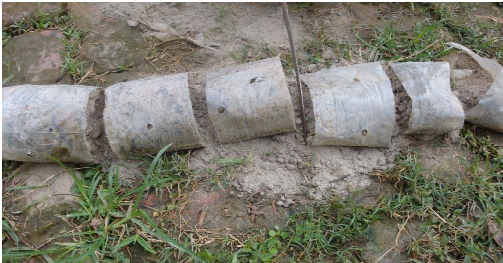
Plate 1.3. Root elongation tube (70 cm) cut into 7 pieces (10 cm/ piece)
