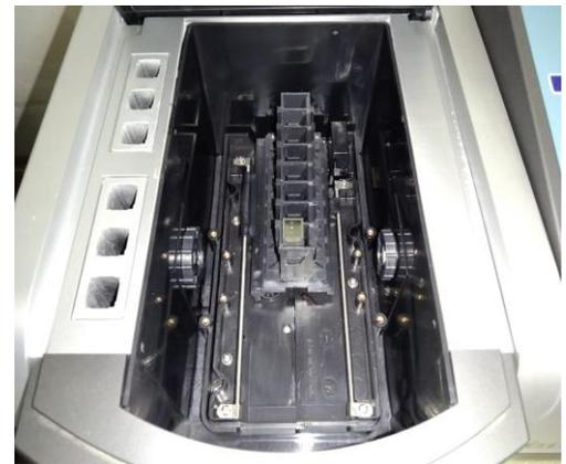
**Placement of glasstubes into spectrophotometer**
