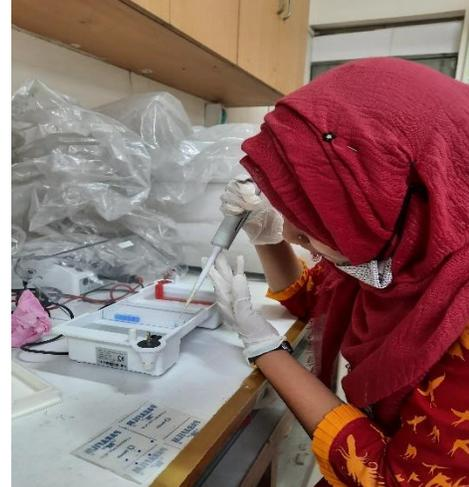
**Figure 6. Placement of loading dye with sample into agarose gel**
