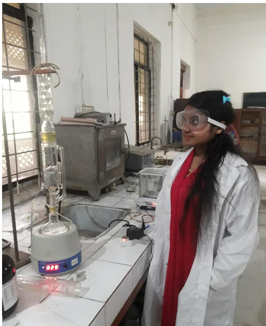
Plate 1. Photograph showing Extraction of rapeseed and mustard oil by soxhlet aparatus.
