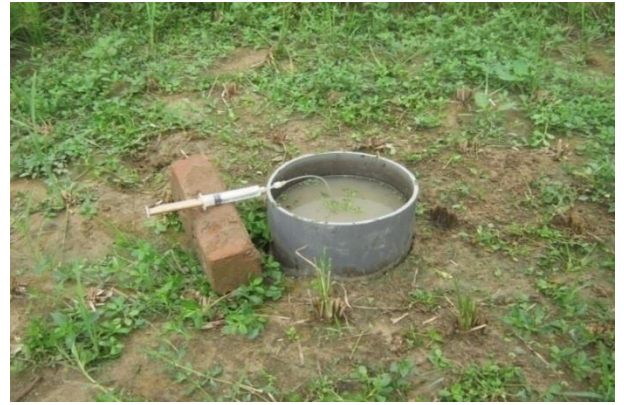
Figure 4.7. Core installed in the middle of a plot and pore-water collection by rhizon sampler from boro rice field
