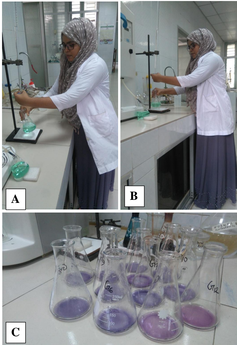
Plate 8. Titration for protein determination. A, B. Titration, C. Color change of the solution after titration .
