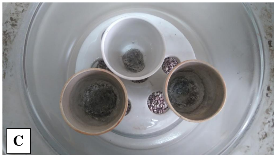
Plate 5. Determination of Ash percentage A. Sample as powdered form for analysis, B. Sample in crucible after dry, C. Sample in crucible after ignition.
