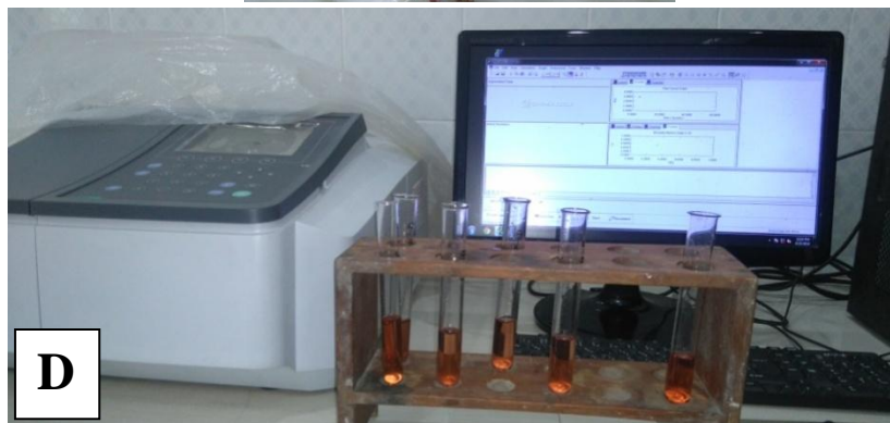
Plate 9. Determination of fat, fiber and iron percentage. A. Fat% determination, B. Fiber% determination, C. Making iron solution, D. Iron% determination by UV-ray machine. and reading was noted from computer.
