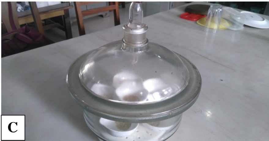
Plate 4. Determination of chlorophyll content and moisture percentage. A. Measurement of chlorophyll content, B. Sample in the basin in desiccator before dry, C, D. Sample in the basin in desiccator after dry.
