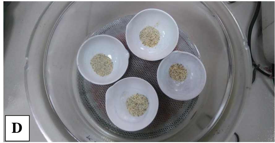
Plate 4. Determination of chlorophyll content and moisture percentage. A. Measurement of chlorophyll content, B. Sample in the basin in desiccator before dry, C, D. Sample in the basin in desiccator after dry.
