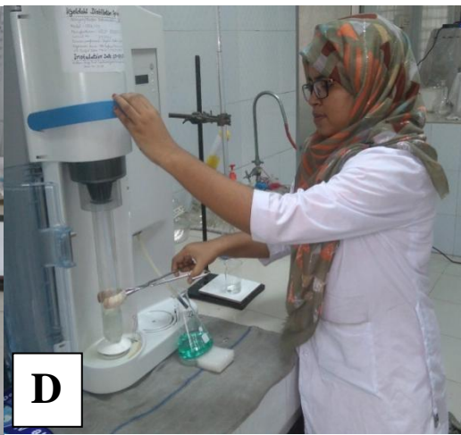
Plate 7. Protein distillation. A. Digested sample in volumetric flask, B. Indicator with boric acid in conical flask, C. Distillation machine, D. Placement of distillation tube with sample in distillation machine.
