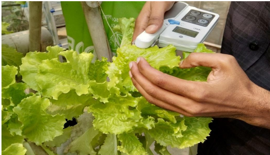
Plate 3. Determination of SPAD value by SPAD plus chlorophyll meter
