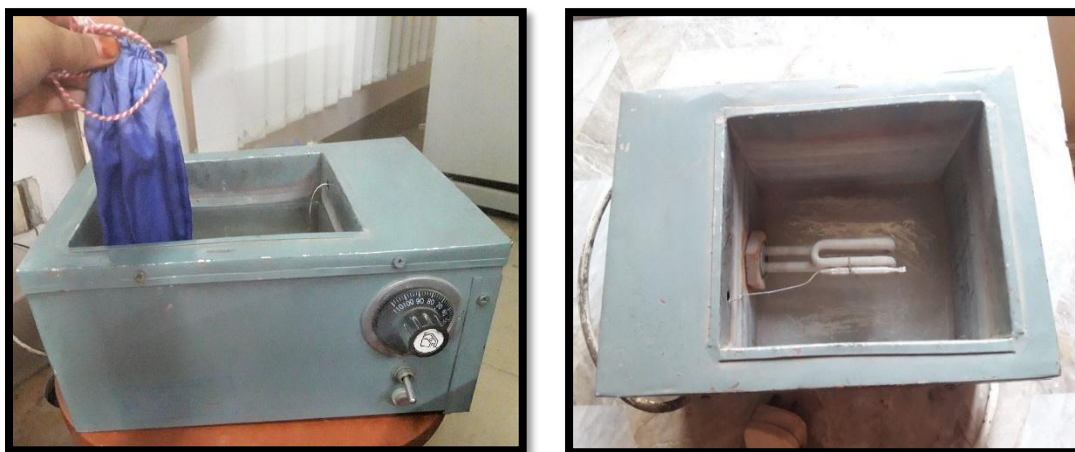
Figure 01: Hot Water Treating Device
