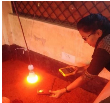
Plate 5: Measuring lux of different color of LED light with lux meter
