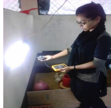
Plate 5: Measuring lux of different color of LED light with lux meter
