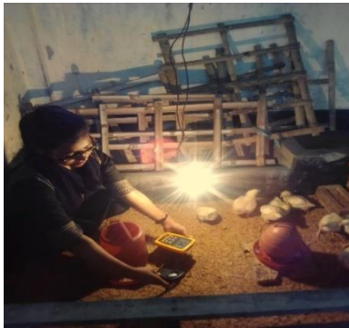
Plate 5: Measuring lux of different color of LED light with lux meter
