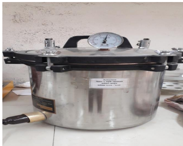
Plate 2: Autoclaving at 121°C by Autoclave machine
