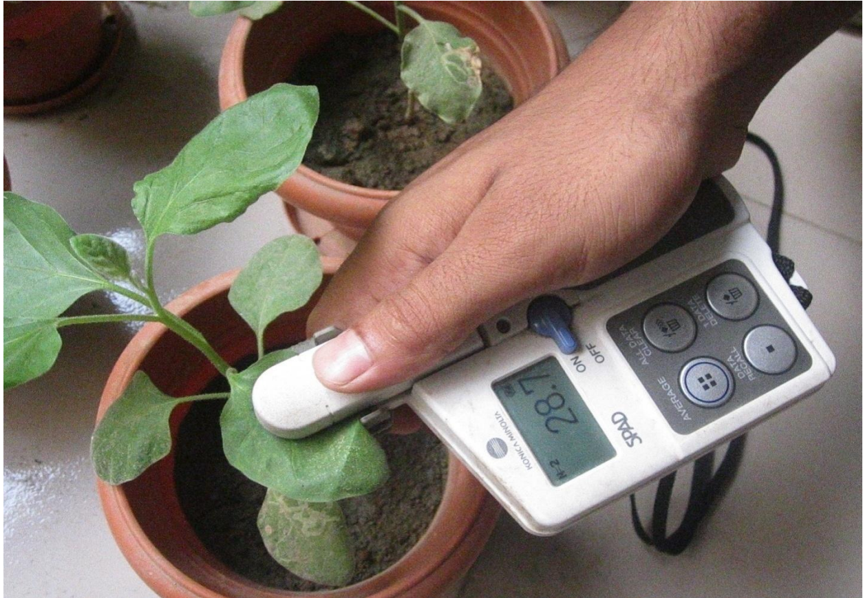
Plate 10. Measurement of Chlorophyll content of Eggplant leaf by SPAD 502 Plus Chlorophyll Meter
