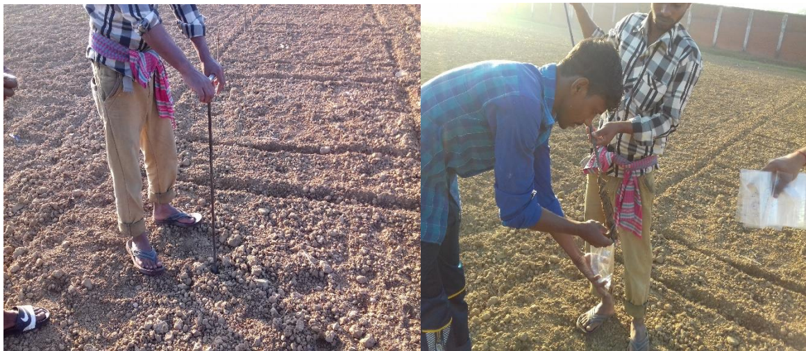
Plate 2. Collection of soil sample for the P^H and Organic Carbon percentage measurement
