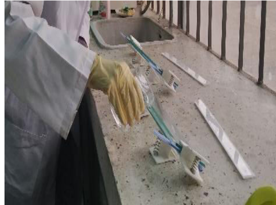
Figure 6. PAGE gel preparation
