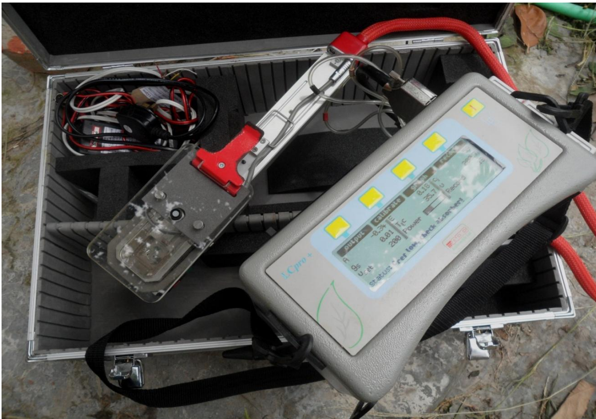
Figure 3. “LC Pro + ” machine used to record the data of physiological features.
