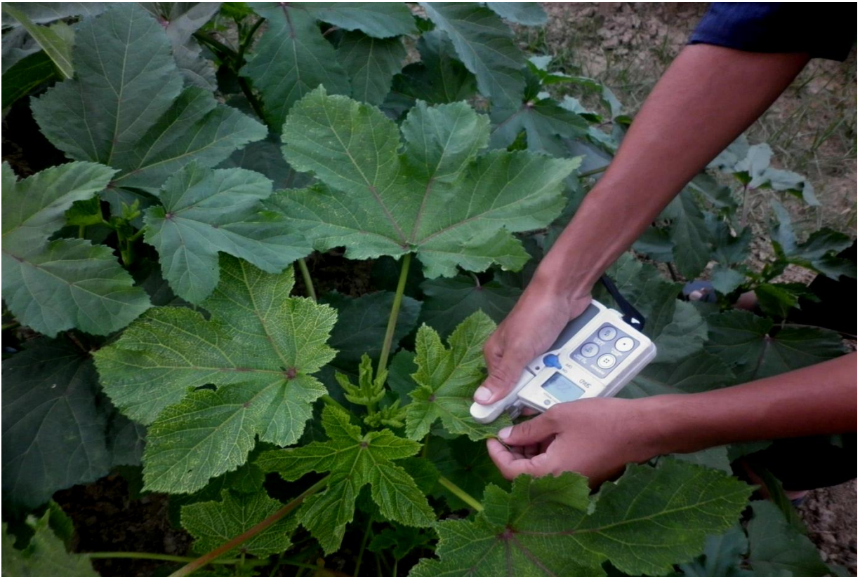
Figure 2. Recording net chlorophyll content in plant leaf by “S-PAD”.
