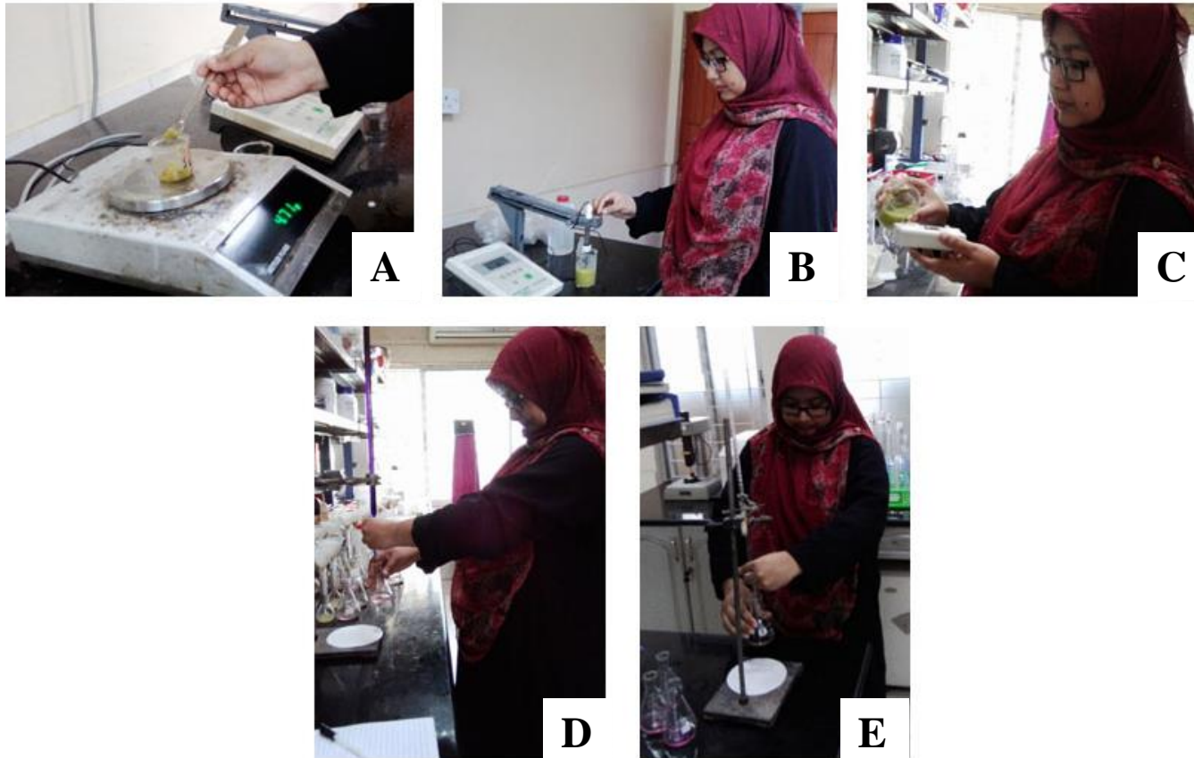
Plate 5. Data collection of different nutritional traits. A) Weighting fruit sample, B) Estimation of fruit pH, C) Estimation of brix percentage, D) Estimation of vitamin-C content and E) Estimation of titratable acid content
