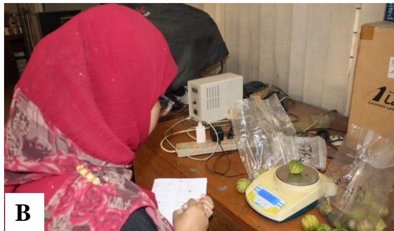
Plate 3. Collection of data. A) Measuring fruit length and diameter using Digital Caliper-515, B) Measuring fruit weight using electric precision balance
