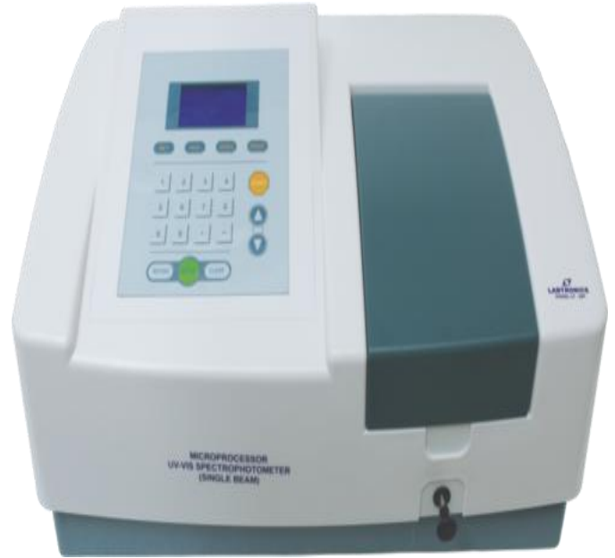
Plate 2. Single Beam UV-VIS Spectrophotometer
