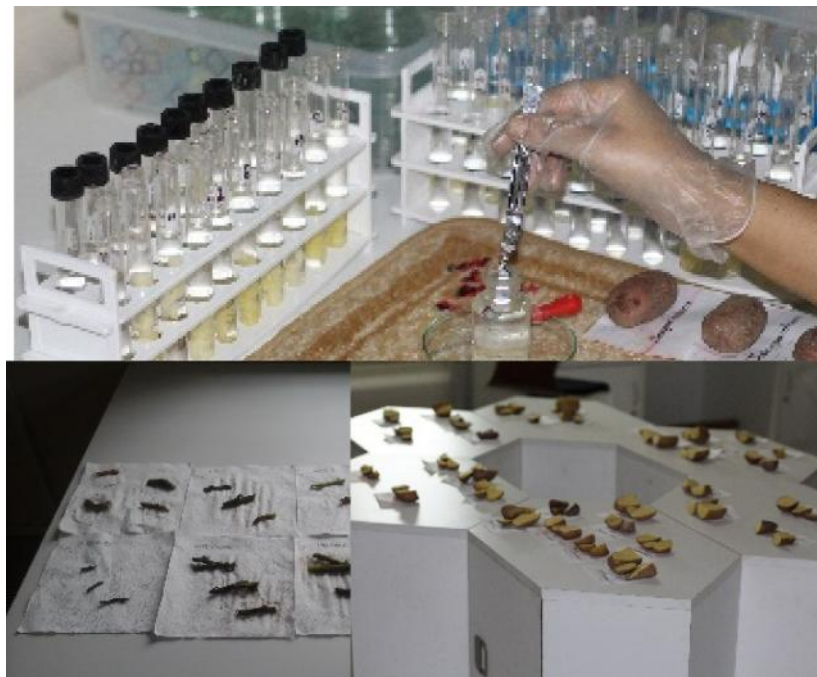
Fig. 3.b. Different steps of samples preparation infected by R. solanacearum isolate and preserve the pathogen in the laboratory.
