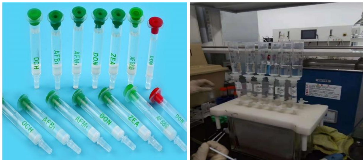
Fig. 2. DON column for Extraction.
