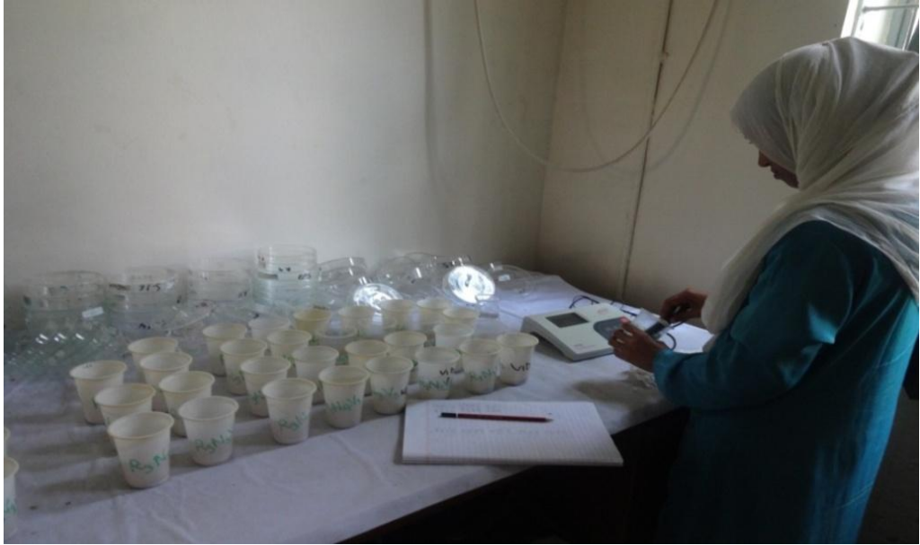
Plate 5. View of the electrical conductivity test of wheat seed after harvest
