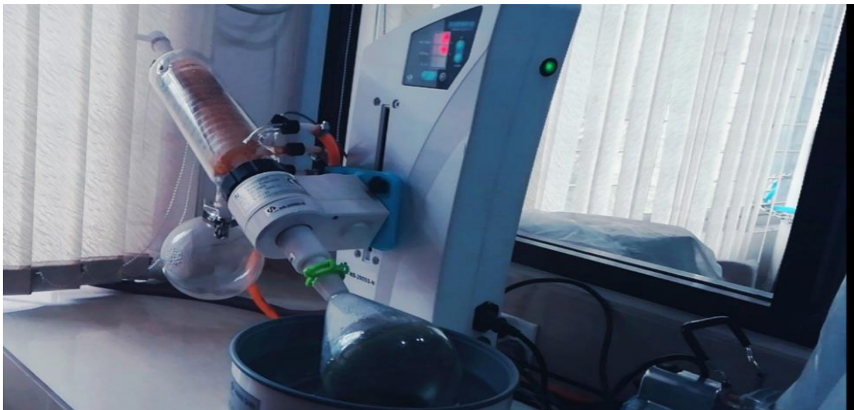
Figure 9: Evaporate the aqueous extract by rotary evaporator (HS-2005S) at 40 0 C for 30 minutes
