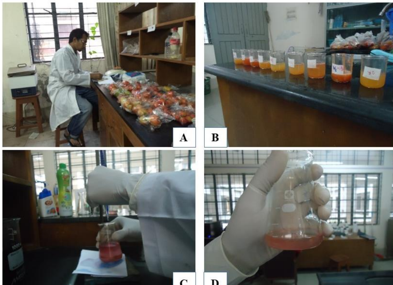
Plate 5: Different types of activities for estimation of vitamin C. A. Measuring the weight of tomato, B. Extraction of tomato juice, C. Titration for estimate vitamin C in tomato, D. Estimation of vitamin C.
