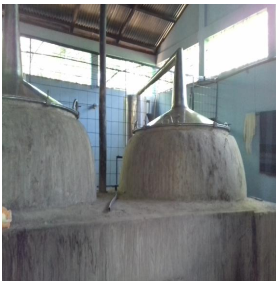
Plate 7: Distillation process of Agar Wood chips
