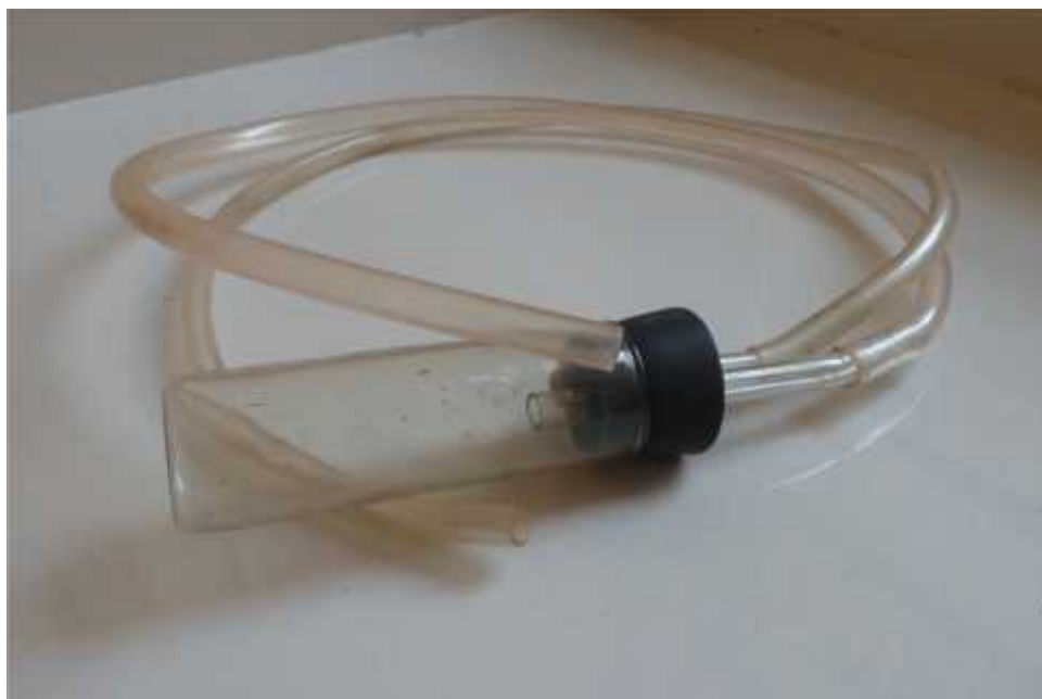
Plate 2. Aspirator for collection of S. cerealella from infested grain
