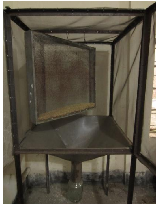
Plate 9. Metallic cage especially made for rearing and facilitating the adult emergence of S. cerealella .
