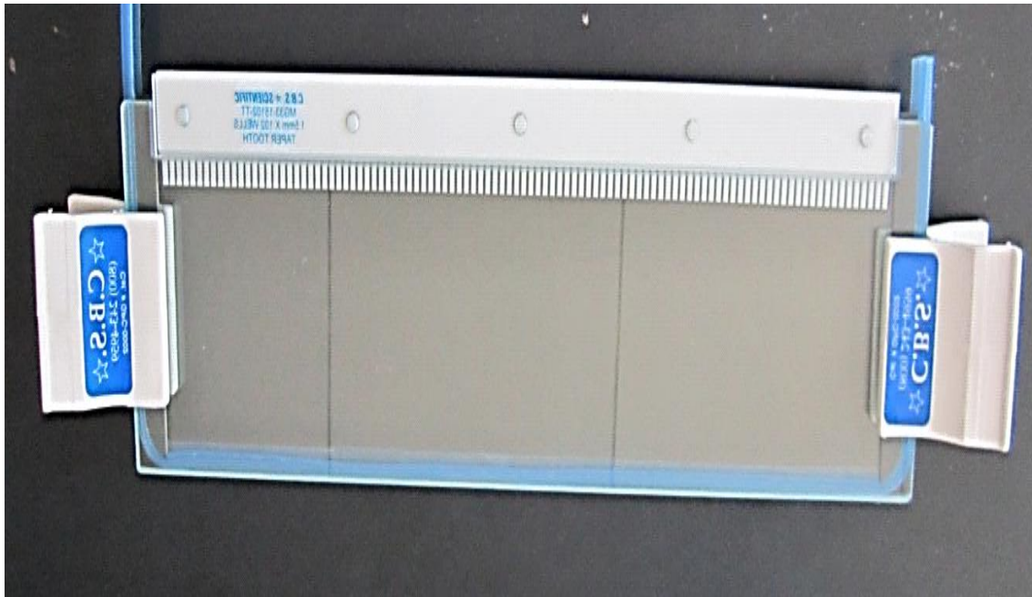
Plate 5. Assembly of glass plates with the comb inserted inside the two glass plates.
