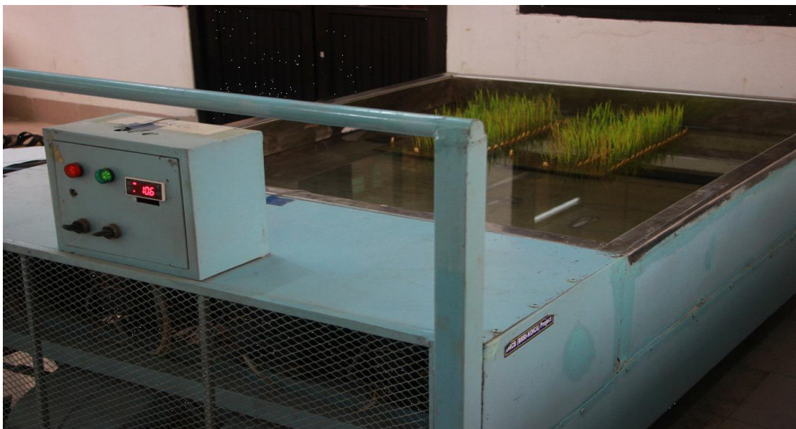
Plate 11. Screening of backcross progenies of BRR1 dhan28XHbj.BVI in cold water tank at 10.6 0 C temperature.
